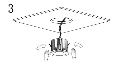
Break the spring upward in the direction indicated by the arrow.
