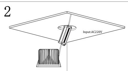
Instruction marked on the driver, and do the insulation protection well. (Standard product input voltage: AC220V 50/60Hz)
