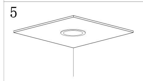
The installation is completed until the frame is flat with the ceiling.
