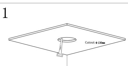
Open the mounting hole on ceiling according to the cutout size, this product is suitable for the thickness of 1-20mm of ceiling.
