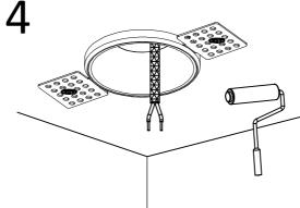
The trimless fixed bracket and joints shall be painted with plaster (it is recommended to paste mesh cloth before plaster to avoid wall cracking), and be covered with smooth and clean.
