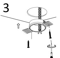
Clip the trimless mounting bracket intothe cutout hole in the ceiling, then lock the trimless mounting bracket to theceiling with self-tapping screws and pull the wire out of the bracket.
