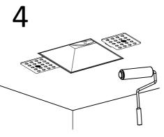
The trimless fixed bracket and joints shall be painted with plaster (it is recommended to paste mesh cloth before plaster to avoid wall cracking), and be covered with smooth and clean.
