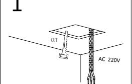
Open the mounting hole on ceiling according to the cutout size, and pass the wires through the hole.
