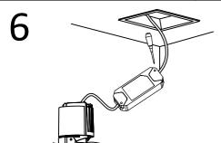
Remove the protective cover of the power supply with a screwdriver, connect the power cord according to the wiring instruction marked on the driver, and do the insulation protection well. And insert the driver into cutout on the ceiling.
