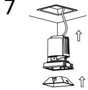
Install the housing on the trimless bracket and make sure it stable, then fix with reflector. Adjustable downlight series can adjust the irradiation angle according to the demand to meet the lighting requirements.
