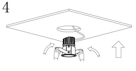
$Press\ the\ mounting\ spring\ upward\ in\ the\ direction\ indicated\ by\ the\ arrow,\ and\ push\ the\ luminaire$ in until the frame is flat with the ceiling.
