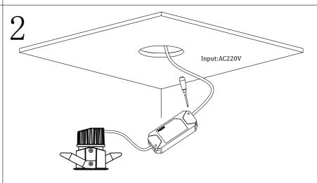
Remove the protective cover of the power supply with a screwdriver, connect the power cord according to the wiring instruction marked on the driver, and do the insulation protection well.
