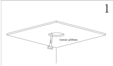
Open the mounting hole on ceiling according to cutout size, this product is suitable for the thickness of the 5-20mm of ceiling
