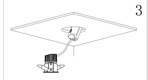
Insert the driver into cutout on the ceiling.
