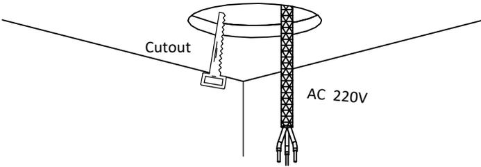
Open the mounting hole on ceiling according to the cutout size.
