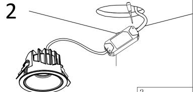
Remove the protective cover of the power supply with a screwdriver, connect the power cord according to the wiring instruction marked on the driver, and do the insulation protection well. And insert the driver into cutout on the ceiling.
