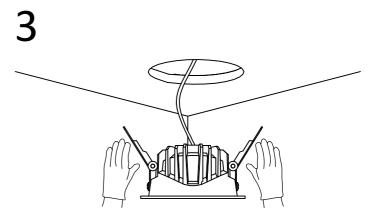
Press the mounting spring into the cutout in the ceiling and push the luminaire in.
