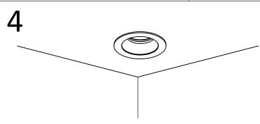
Turn on the power supply, lights up. Warning: The fitting should be never covered by insulation gasket or similar materials under any circumstance. Please ensure that the wires are conneced correctly before turning on the power supply. Do not look emitting lights directly
