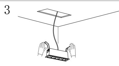
Remove the protective cover of the power supply with a screwdriver, connect the power
