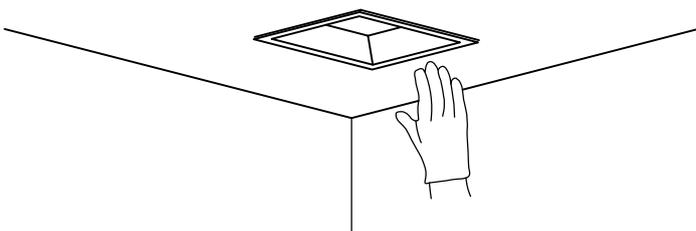
The installation is completed until the frame is flat with the ceiling.
