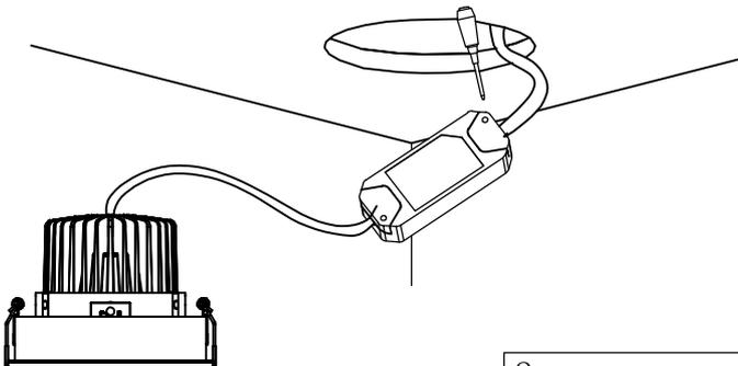
Remove the protective cover of the power supply with a screwdriver, connect the power cord according to the wiring instruction marked on the driver, and do the insulation protection well. And insert the driver into cutout on the ceiling.
