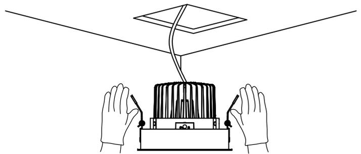
Press the mounting spring into the cutout in the ceiling and push the luminaire in.
