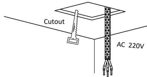
Open the mounting hole on ceiling according to the cutout size.
