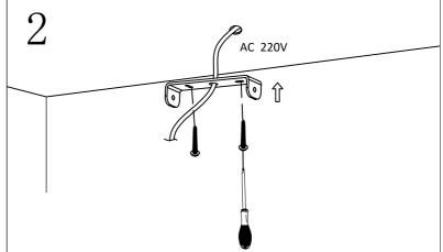
Thread the wire through the hole of bracket, and fasten the bracket with screws on the ceiling.
