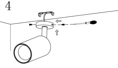
Insert the extra wire into ceiling first, then fix the fitting on the bracket with screws.
