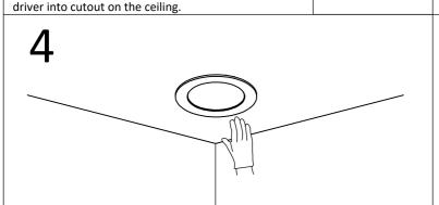
The installation is completed until the frame is flat with the ceiling. Adjustable downlight series can adjust the irradiation angle according to the demand to meet the lighting requirements.
