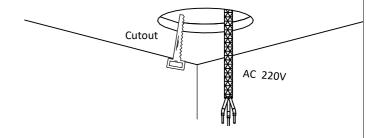
Open the mounting hole on ceiling according to the cutout size, and pass the wires through the hole.
