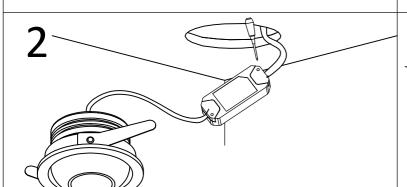
Remove the protective cover of the power supply with a screwdriver, connect the power cord according to the wiring instruction marked on the driver, and do the insulation protection well. And insert the driver into cutout on the ceiling.
