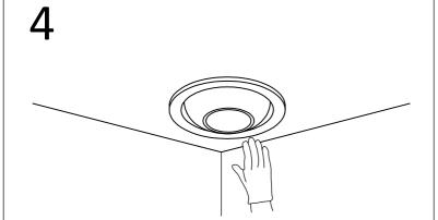
The installation is completed until the frame is flat with the ceiling. Adjustable downlight series can adjust the irradiation angle according to the demand to meet the lighting requirements. 5 Turn on the power supply, lights up.
