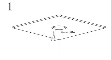
Open the mounting hole on ceiling according to the cutout size, this product is suitable for the thickness of 1-30mm of ceiling.
