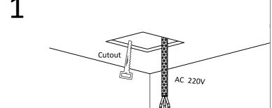
Open the mounting hole on ceiling according to the cutout size.
