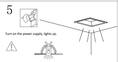
Warning: The fitting should be never covered by insulation gasket or similar materials under any circumstance.
