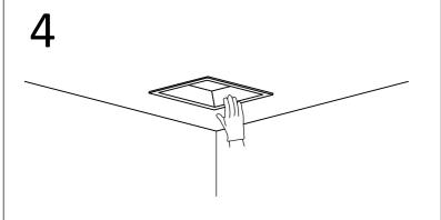
The installation is completed until the frame is flat with the ceiling. Adjustable downlight series can adjust the irradiation angle according to the demand to meet the lighting requirements.
